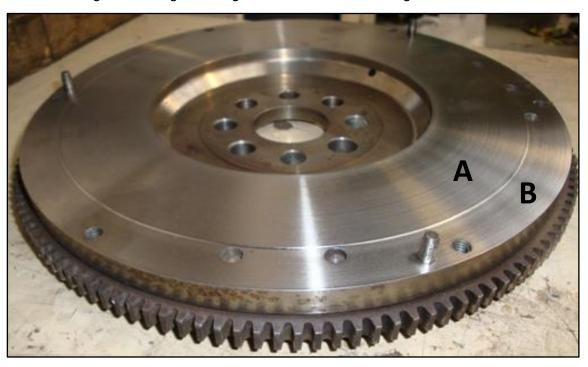
M40 Minimum of 22.7mm on the inner surface. (Point A)
