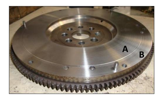
M40 Minimum of 22.7mm on the inner surface. (Point A)
